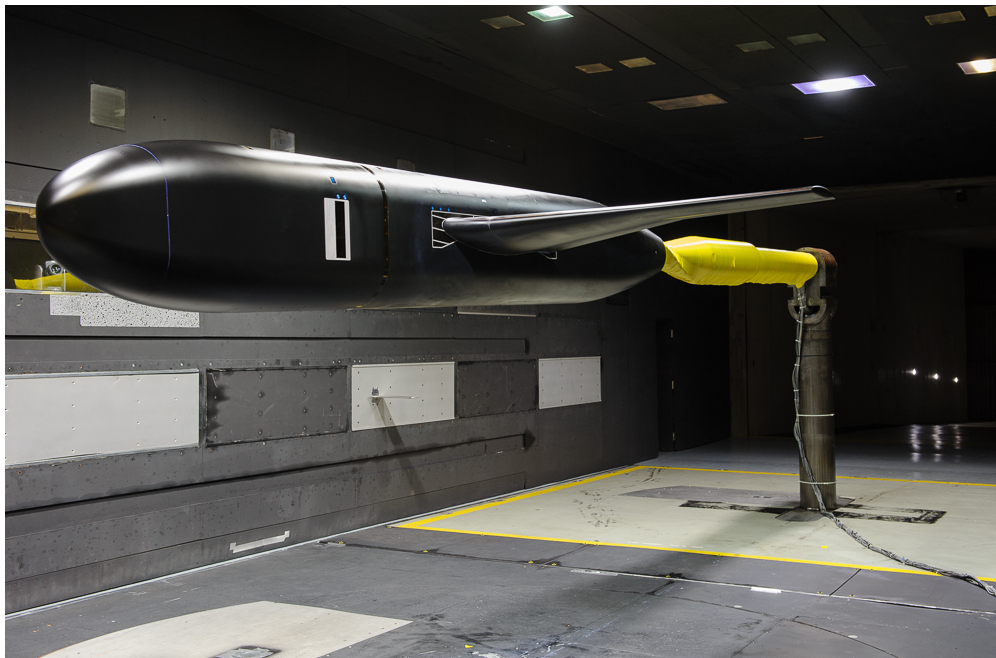
Figure 2: Port-side image of the wing-fuselage junction model installed in the 14- by 22-Foot Subsonic Wind Tunnel.
