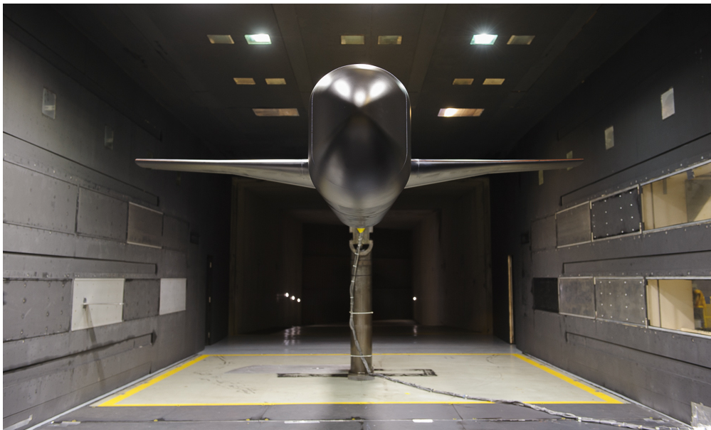
Figure 4: Front-view image of the wing-fuselage junction model installed in the 14- by 22-Foot Subsonic Wind Tunnel.
