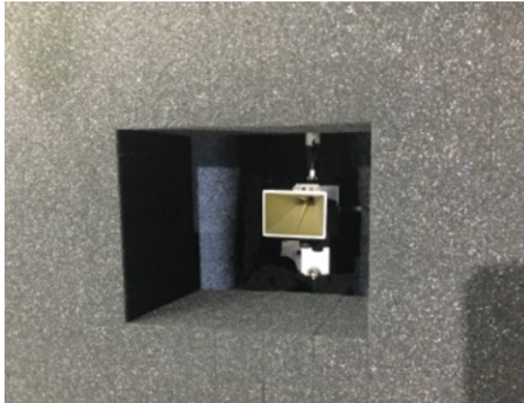
Figure 2. Test Configuration 3 showing the SAS-574 Antenna and Polyethylene Foam Support Enclosure.
