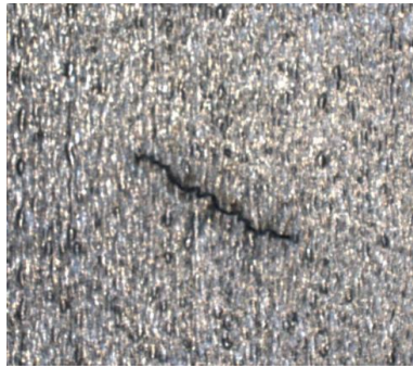
Laser cut crack
