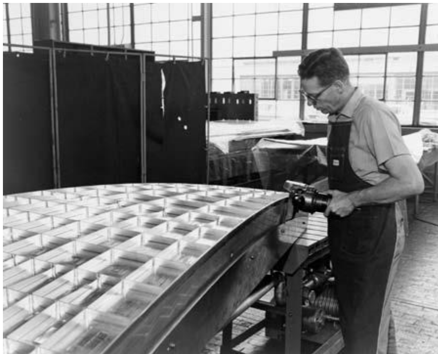
Figure 2. Large plate with integrally machined stiffeners. NASA photo 1966-02109L.
