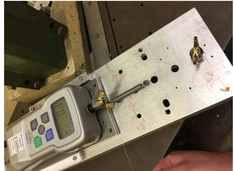
Testing of Kevlar/epoxy joints
