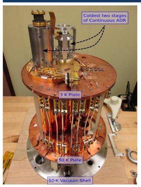
10 current leads needed to run the 4 CADR stages and the superconducting heat switch between Stages 1 and 2
