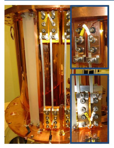
In the new cryostat, it was decided to try spanning 50 to 3 K using a single tape per circuit leg
