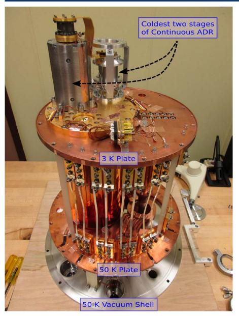
A cryostat was built to contain a 4-Stage Continuous Adiabatic Demagnetization Refrigerator (CADR).
