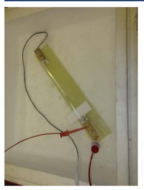
There was a fear that a rapid pumpout of the Dewar flexed the HTS tapes and broke the YBCO layer
