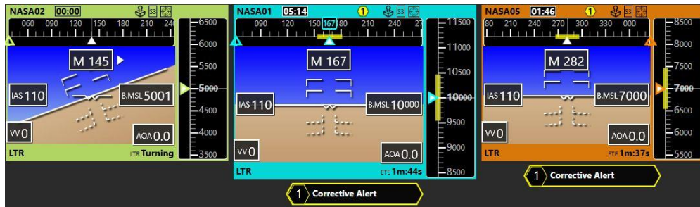
Fig. 1 A view of the baseball cards in the 1:3 control condition during a multi-threat event. Active DAA alert status and maneuver guidance are visible as part of the baseball card of the focused (middle) and unfocused UA (right). The stopwatch (top) was used to manually track time on task during supervisory missions.
