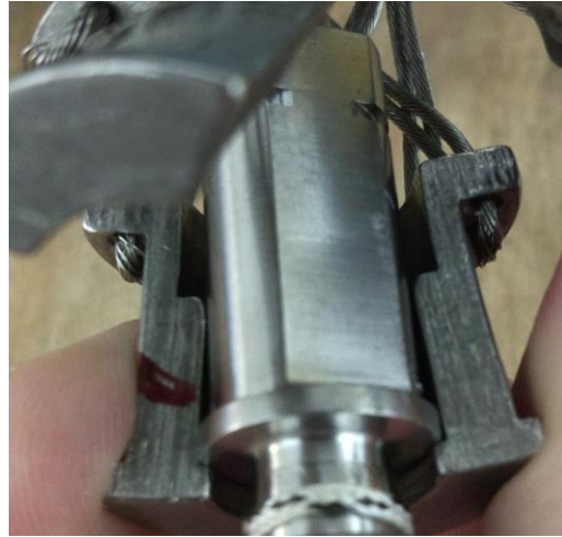
Figure 8. Position of collar in Kellem after slippage. Image credit: Joseph Dziekan, NIFS intern.
