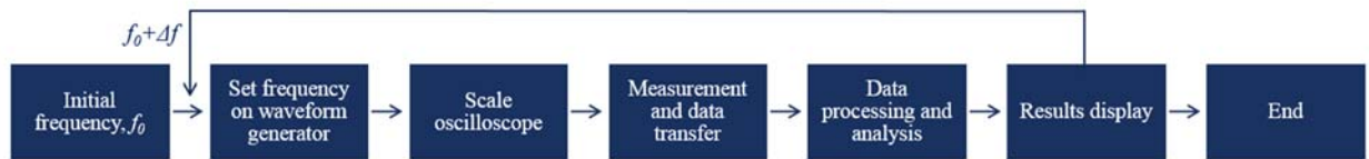
Figure 4. Automated algorithm for data collection and analysis of guided waves for in-process cure monitoring.
