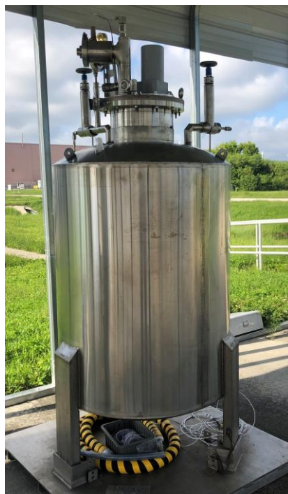
Figure 1. Cryostat with 400-liter vessel and integrated cryocooler for LNG studies.
