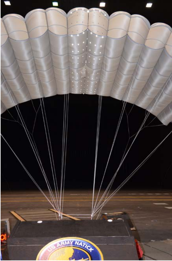
Fig. 4 Inflated canopy showing targets on centerline cell.
