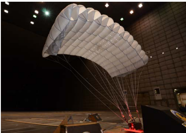
Fig. 3 Installation of ram-air parachute in test section.
