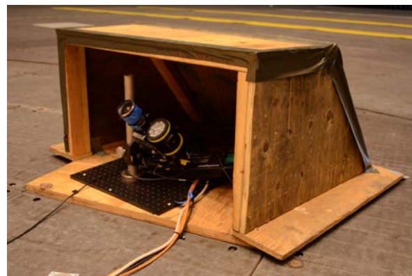
Fig. 7 Upstream floor-mounted canopy camera and lamp. Flow direction is top-right to bottom-left.
