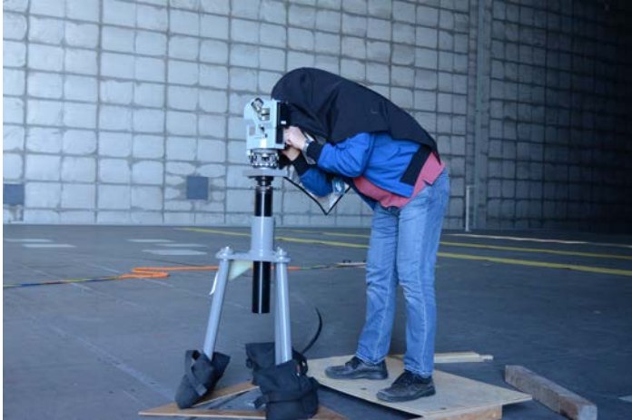
Fig. 8 Measuring ceiling calibration targets with a theodolite.
