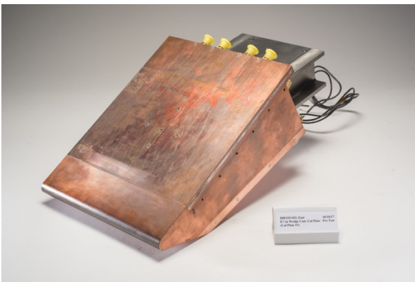
(a) wedge model, water-cooled calibration plate
