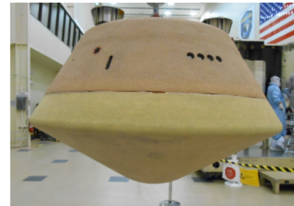
OSIRIS-REx forebody TPS. (~0.8m diameter)
