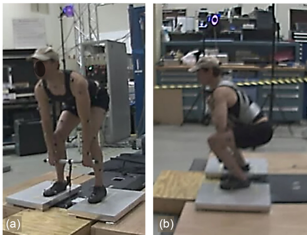
Figure 1.—Hybrid Ultimate Lifting Kit (HULK) device. (a) Configured for single-cable deadlift with T-bar operation. (b) Configured for squat with harness operation.
