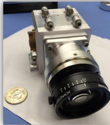
Fig. 2 The JPL OCO-3 camera that will fly on the NEA Scout mission may be upgraded by adding a filter wheel to enhance science return for NME.
