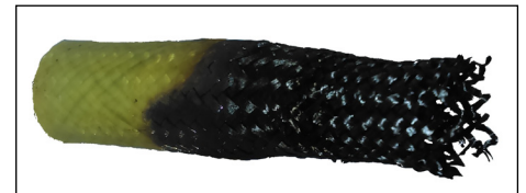
Figure 1. Kevlar sample exposed until demise.
