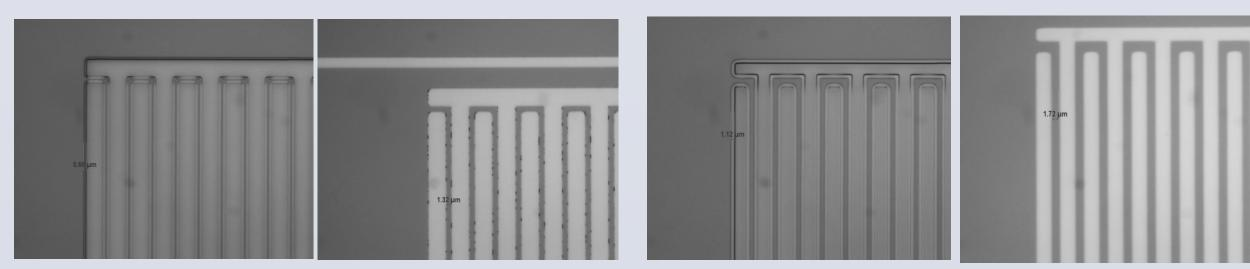
Wafer 5: 1 min 35 s development in MF319 resulted in ~1 -Wafer 1: ~0.65-0.7 um undercut. Undercut was insufficient 1.15 um undercut. Pretty clean but flags in a few spots. As
