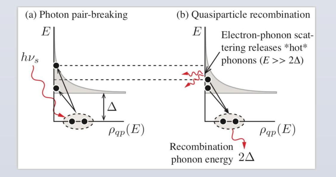
The energy resolution of state-of-the-art photon counting KIDs is nearly an order of magnitude below the statistical (Fano) limit for a pair-breaking device. We have added a meta-material phononic crystal that reduces the loss of recombination and athermal phonons from a KID. The phononic crystal
