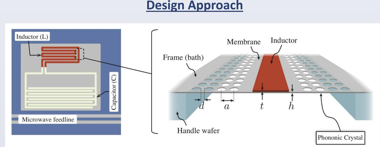
\* Phononic crystal pattern encapsulates inductor (see text for details) \*\* Inductor is low- $T_c$  superconducting thin-film, e.g. Hf ( $T_c \sim 400$  mK) \*\*\* Capacitor is high- $T_c$  superconducting thin-film, e.g. Nb ( $T_c \sim 9$  K)
