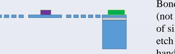
Bond wafer with wax to a handle wafer (not shown). Pattern handle wafer side of silicon wafer and deep reactive ion etch to create membrane. Remove handle wafer by dissolving wax.
