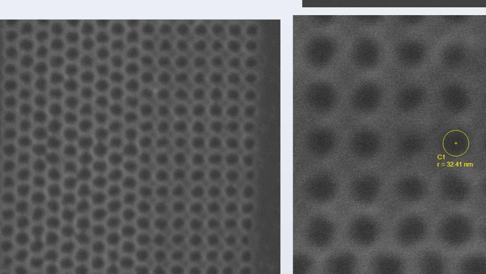
SEM micrographs of etched silicon phononic structures. The silicon is patterned using ZEP 520 resist spun at 2.5krpm, in a Zeiss 100kV with 500uC/cm<sup>2</sup> dose. The features are designed as 60 nm diameter circles and exposed as polygons rather than as zero dimensional spots to give approx 64 nm diameter as fabricated holes on a 110 nm pitch. Phononic pattern consists of both hexagonal and square tiling.
