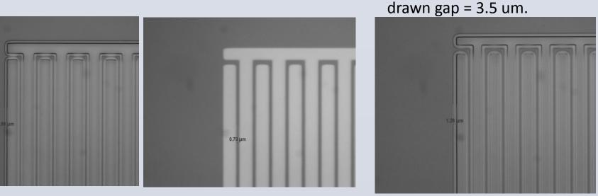
Wafer 2: 1 min 40 s development in MF319 resulted in ~1 – 1.15 um undercut. Pretty clean but flags in a few spots. Delamination occurring b/c 2.5um gap too small to support resist.
