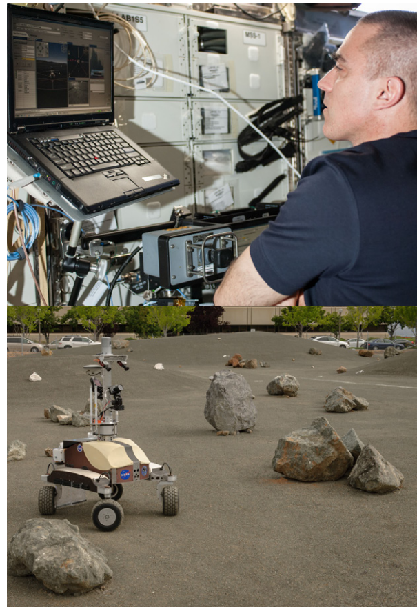
Figure 8. Top: Astronaut Chris Cassidy remotely operating K10 from the ISS (ISS036-E-008908), bottom: K10 performing site survey using on-board cameras and instruments (Phase 1).
