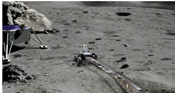
Figure 1. Artist's impression of teleoperated rover on lunar farside deploying a polyimide antenna.
