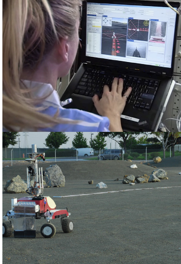
Figure 10. Top: Astronaut Karen Nyberg remotely operating K10 from the ISS, bottom: K10 documenting a deployed polyimide antenna arm (Phase 3).
