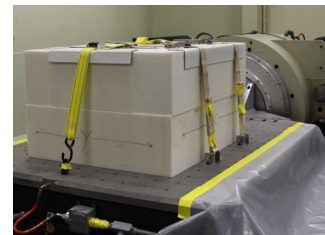
Figure 3. Foam-Mounted Flight Acceptance Vibration Test.
