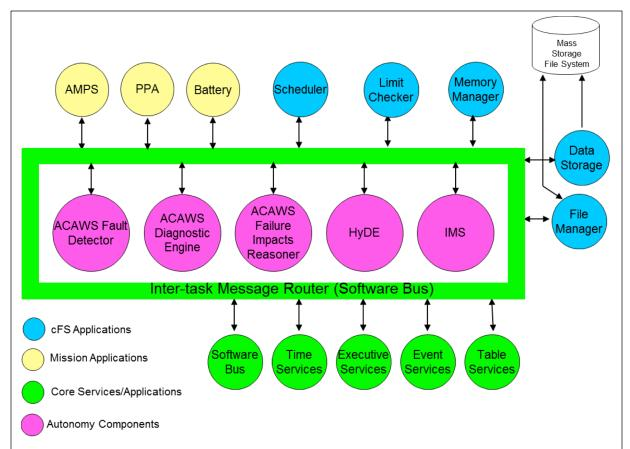
Figure 1 – The autonomy applications, the primary services provided by cFS, a set of common reusable cFS applications, and the representative spacecraft subsystems perform integrated spacecraft functions in a flight-like software environment
