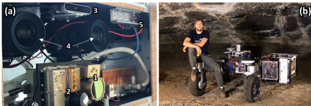
Figure 1-a. Cave instrument package consisting of point spectrometers (1), a multi-illuminant spectral imager (2), a 3D depth mapping sensor (3), stereo DSLR cameras (4), and custom photographic illumination (5). Figure 1-b. The CaveR rover used to carry the science payload and simulate a NASA planetary cave mission.
