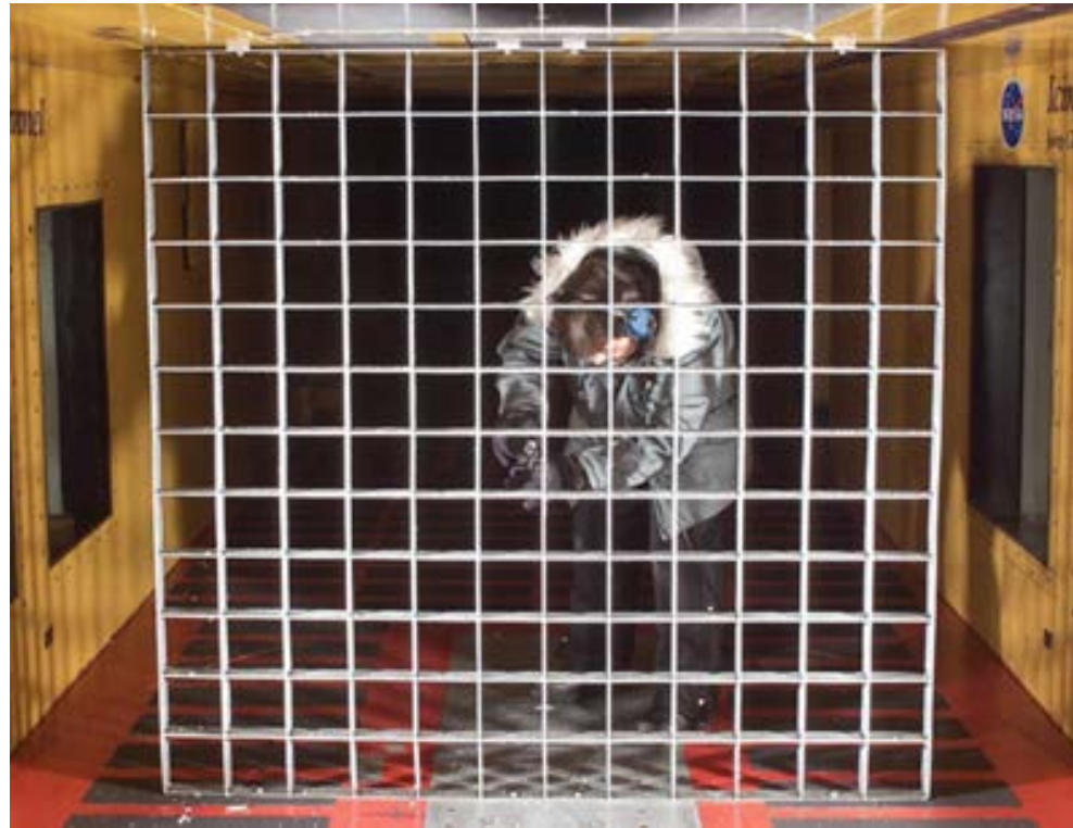
Technician measuring the thickness of ice accreted on the Grid.
