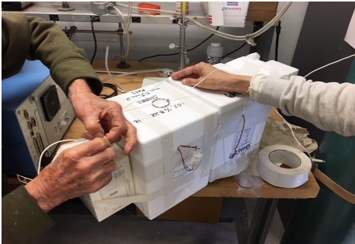
Preparation of "parallel" ozonesonde (two radiosondes, two ozonesondes) at NASA/WFF in June 2018
