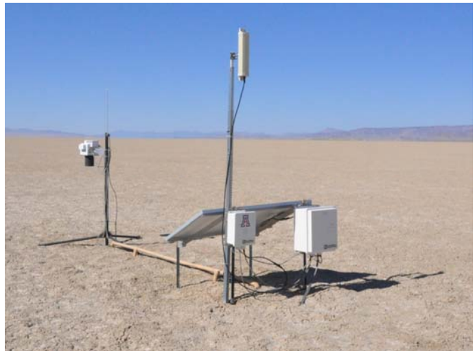
Fig. 1. GVR at Railroad Valley, including the solar panel for charging, electronics boxes, and Wi-Fi antenna. The focal plane of the GVR is 1.5 m above the ground.
