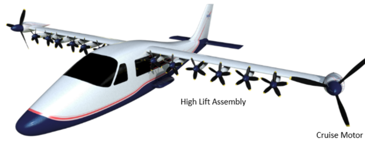
Fig. 1 Rendering of the X-57, depicting the inboard high lift assembly and the larger cruise motors located on the wing tips
