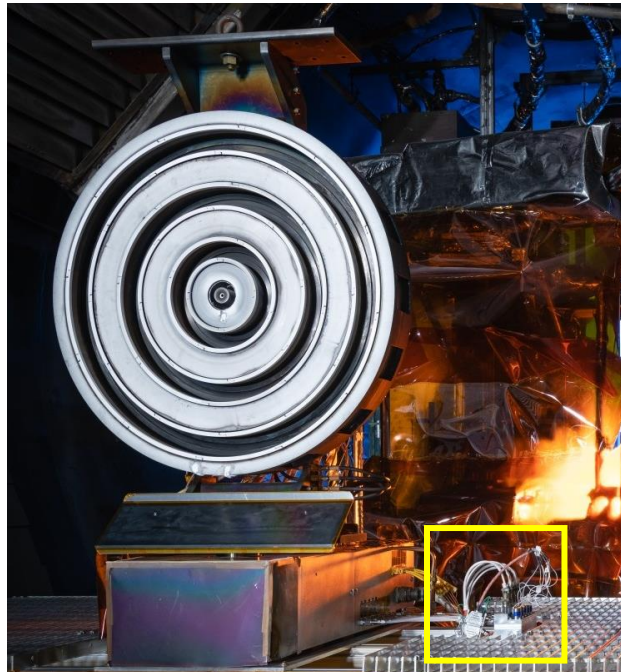
Fig. 4 X3 Nested Hall Thruster (left) and Mass Flow Controller (squared right) inside the vacuum chamber.
