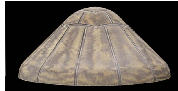
HEEET – Engineering Test Unit (1 m dia)
