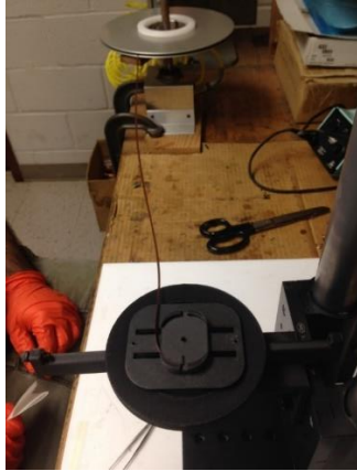
Figure 12. Superconducting coil winding
