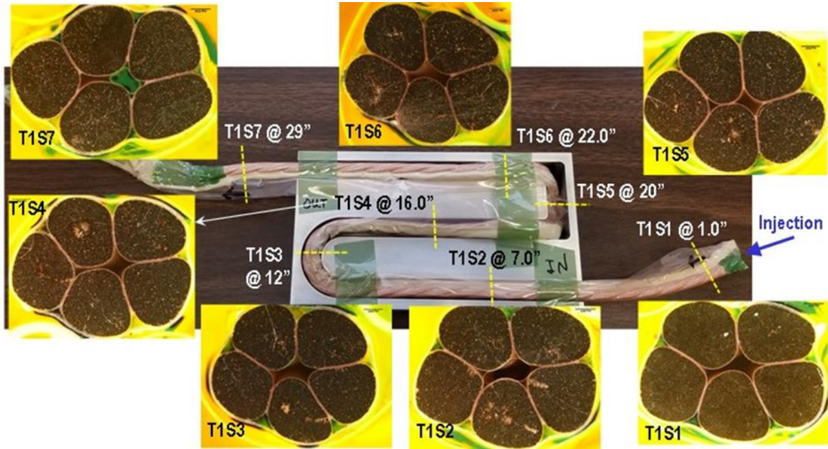
Figure 9. Anatomy of VaAIP processed Litz1 wire.
