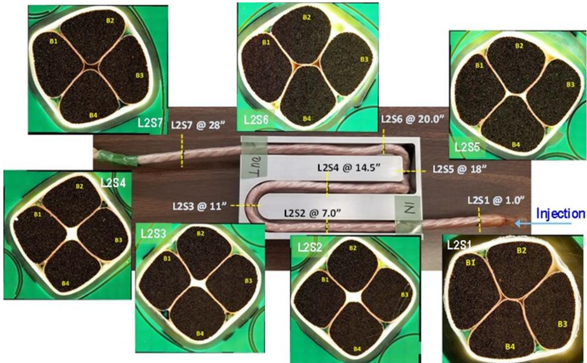
Figure 10. Anatomy of VaAIP processed Litz2 wire.
