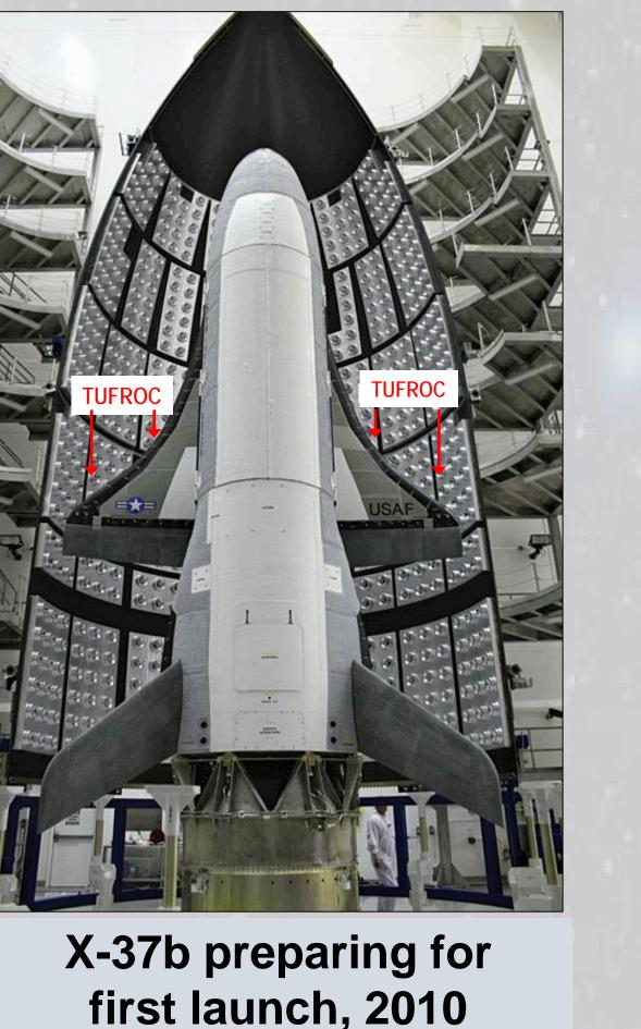
The TUFROC wing leading edge has successfully flown and reentered on four missions with X37B, with a fifth flight currently underway
