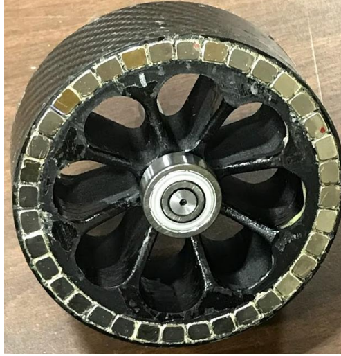
Figure 6 Sun gear of PT-2 with its carbon fiber magnet retaining hoop and 0.5 mm walls between magnets.
