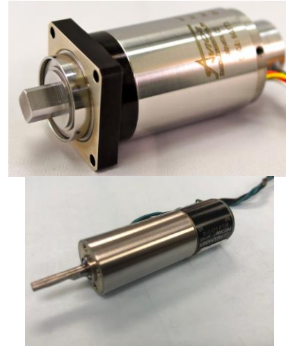
Fig. 10. Approximate sizes of qualified flight (top) and unqualified stepper motor.
