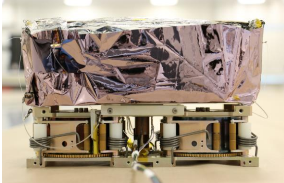
Fig. 5. As-tested solar sail deployer
