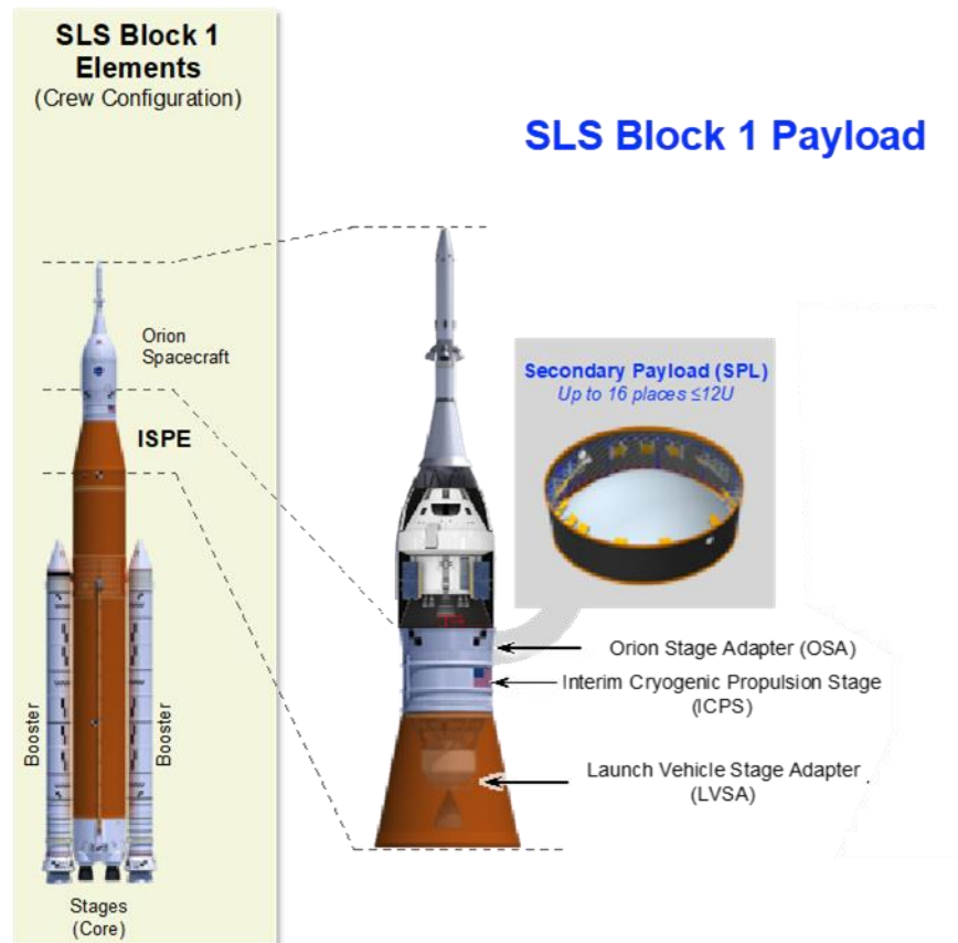
Figure 2 SLS Block 1 Integrated Spacecraft/Payload Element (ISPE)
