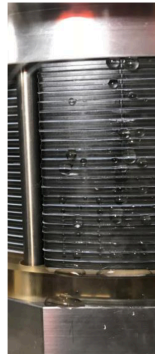
Figure 13. Water Leakage of the Cell Stack at 1,000 psig
