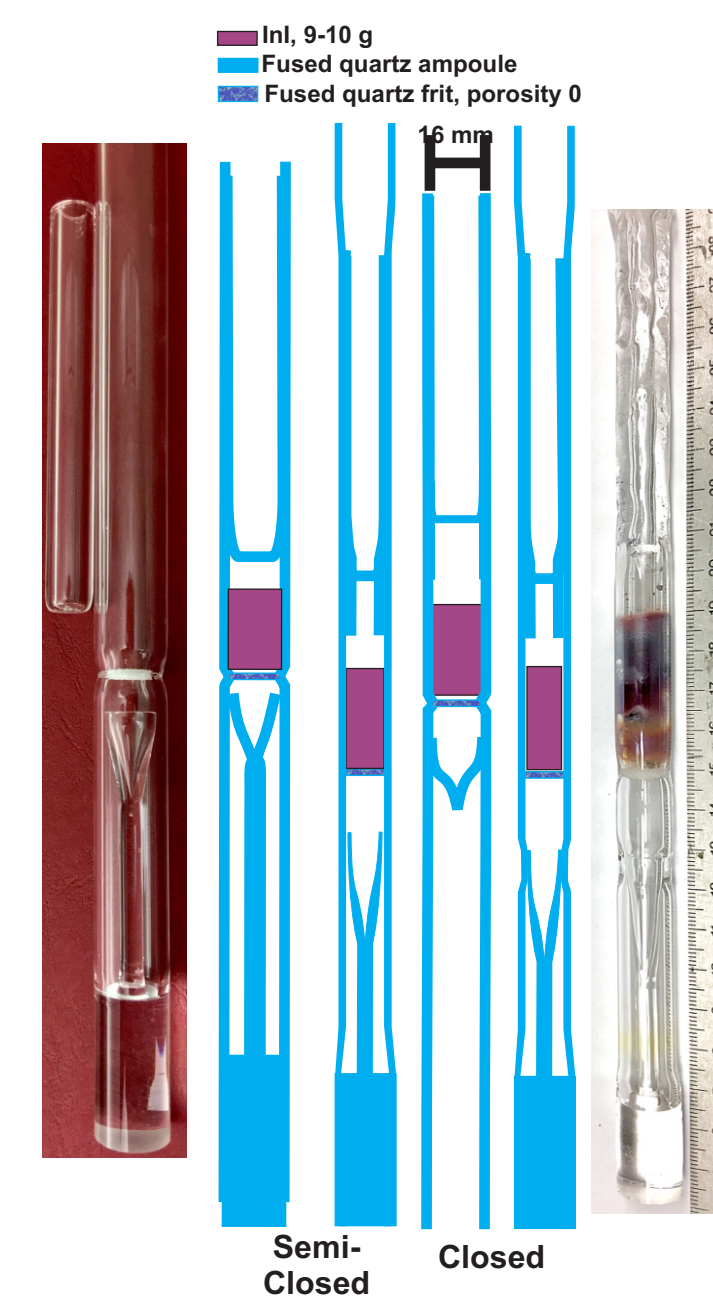
Fig. 2: Vapor growth ampoule designs.
