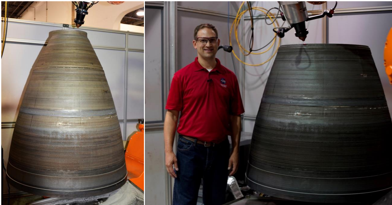
Figure 1. Example of large scale blown powder DED part fabricated in JBK-75 (approx. 44" dia).
