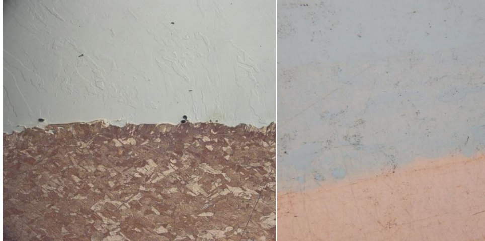
Figure 13. Characteristic Interfaces of the Monel 400 direct to C-18150 using LWDC during development. (Left) Etched Micrograph and (Right) Unetched.
