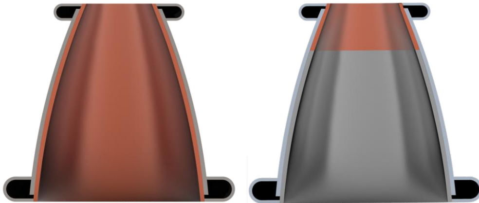
Figure 2. (Left) Example of radial bimetallic configuration and (Right) Axial/Radial Bimetallic/Multi-metallic CWN Configuration.
