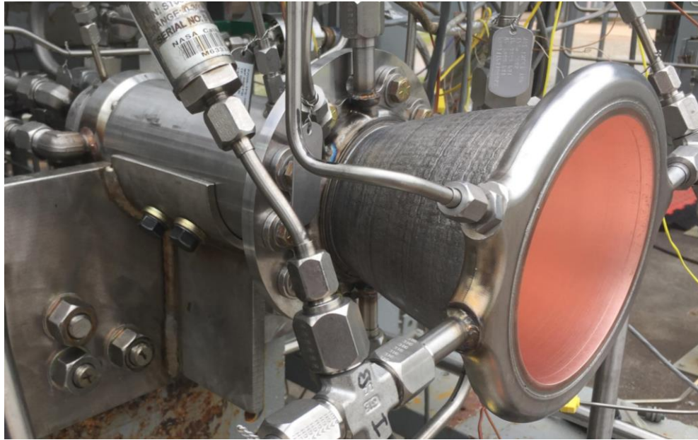
Figure 14. Test configuration with LWDC Bimetallic Nozzle shown at MSFC TS115.
