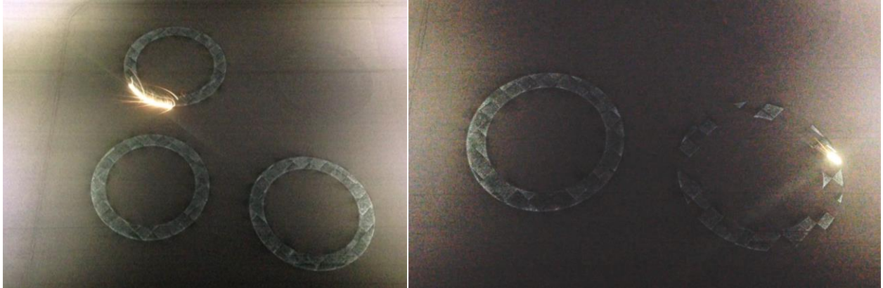
Figure 1. SLM GRCop-84 Chamber Fabrication showing the (Left) Contouring Pass and (Right) In-fill Pass.
