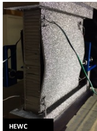
Failed HEWC Coupon
