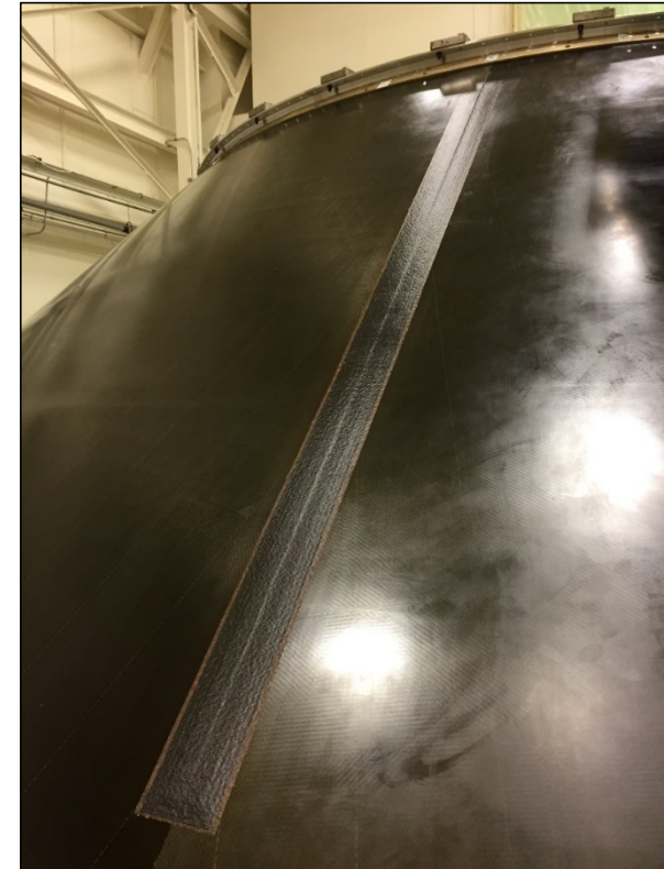
Full-length OML doubler (via scarf joint between 2 segments) after cure
