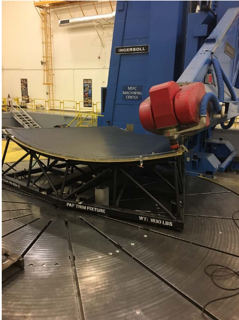
NC Trimming at MSFC
