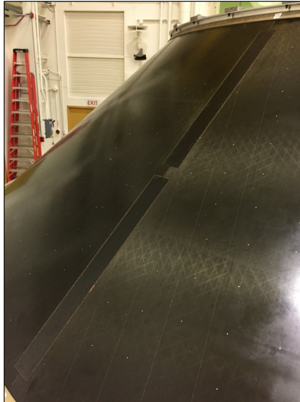
Segmented OML doubler after cure
