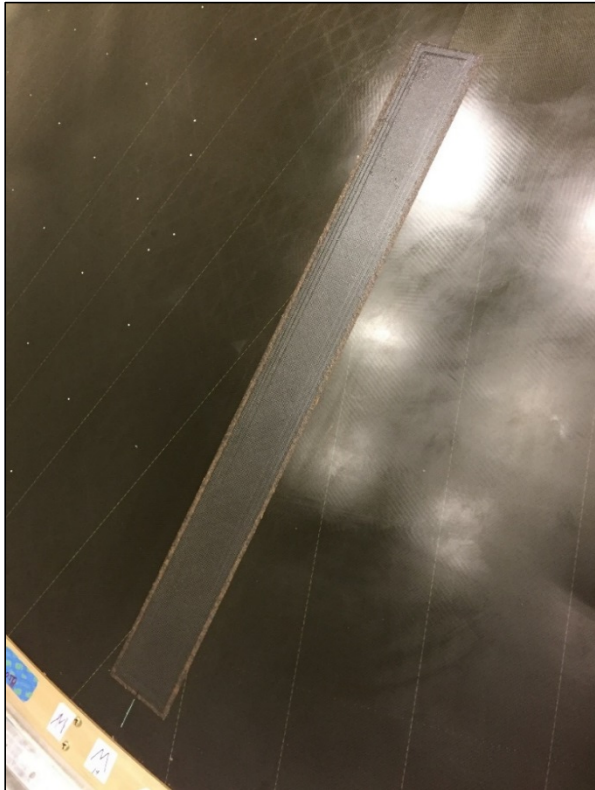
Aft doubler segment (on OML) after cure
