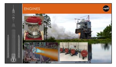
**Basics:** 4 RS-25 engines vs 3 for shuttle, 109% thrust vs 104.5%, new controller and software and nozzle insulation, more than 500,000 lbs thrust each, more than 1 million seconds total ground and flight time. Program starts with 14 flown engines and 2 new serial number engines built from spares.
