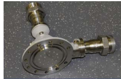
Subscale Integral injector manufactured with SLM. [2]
