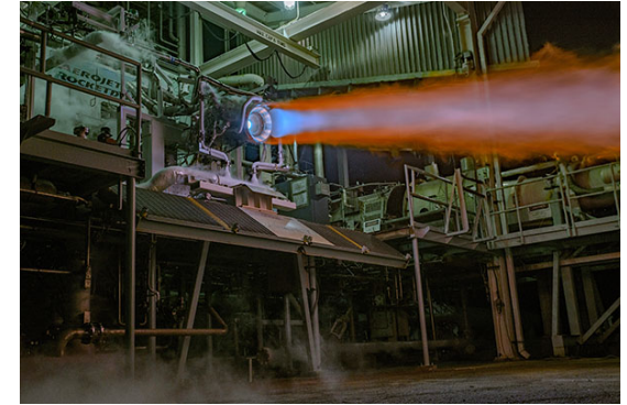
Hot-fire testing of an Aerojet Rocketdyne RL 10C-X prototype engine with 3-D printed core components. [1]
