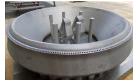
SLM produced integrated nozzle film coolant ring designed and tested at NASA. [3]
