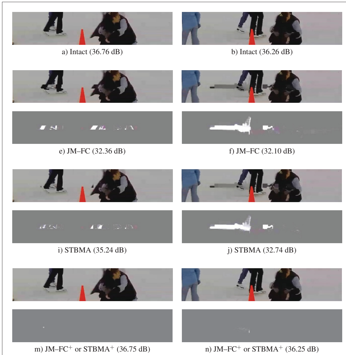
Figure 3.11 Visual comparison of a reconstructed frame in Ice sequence at QP=37 for different methods. In this case, the one bit error occurred in frame 38, slice 15 and on the coeff_token syntax element. The received corrupted packet satisfies the two conditions (it is decodable and the number of decoded MBs is correct (44 MBs)). The pictures on the left side of the figure are showing the reconstructed frame 38 by different approaches. In each case, the difference from intact are also captured by stream analyzer and provided. The pictures on the right side of the figure are showing the error propagation in each case. In fact, twenty frames after the corrupted frame, frame 59 is captured to demonstrate the effect of the error on the following frames.
