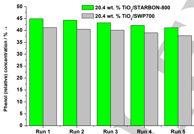
Figure 7. Multi-cycle performance of 20.4 wt. %TiO 2 /STARBON-800_48 μm and 20.4 wt. %TiO 2 /SWP700_48 μm photocatalysts in degradation of phenol in aqueous
