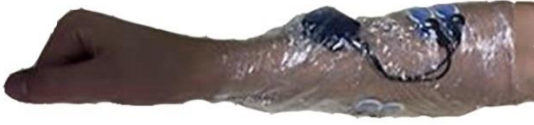
Figure 1: Electrodes placed on the FDS and ECRB forearm muscles with transmitters secured to the forearm using Plastic Wrap Cling Film (UK) (Image from Participant 6).
