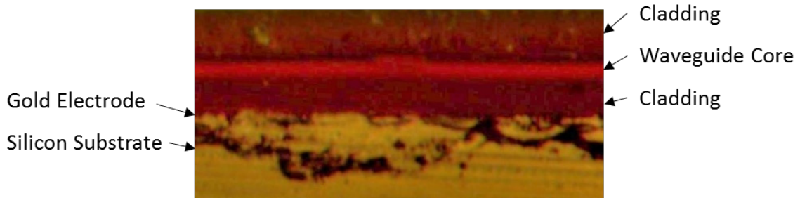
Figure 4.4 Vertical cross-section of a rib waveguide structure fabricated with a polycarbonate core layer exhibiting a cleanly diced waveguide end face.
