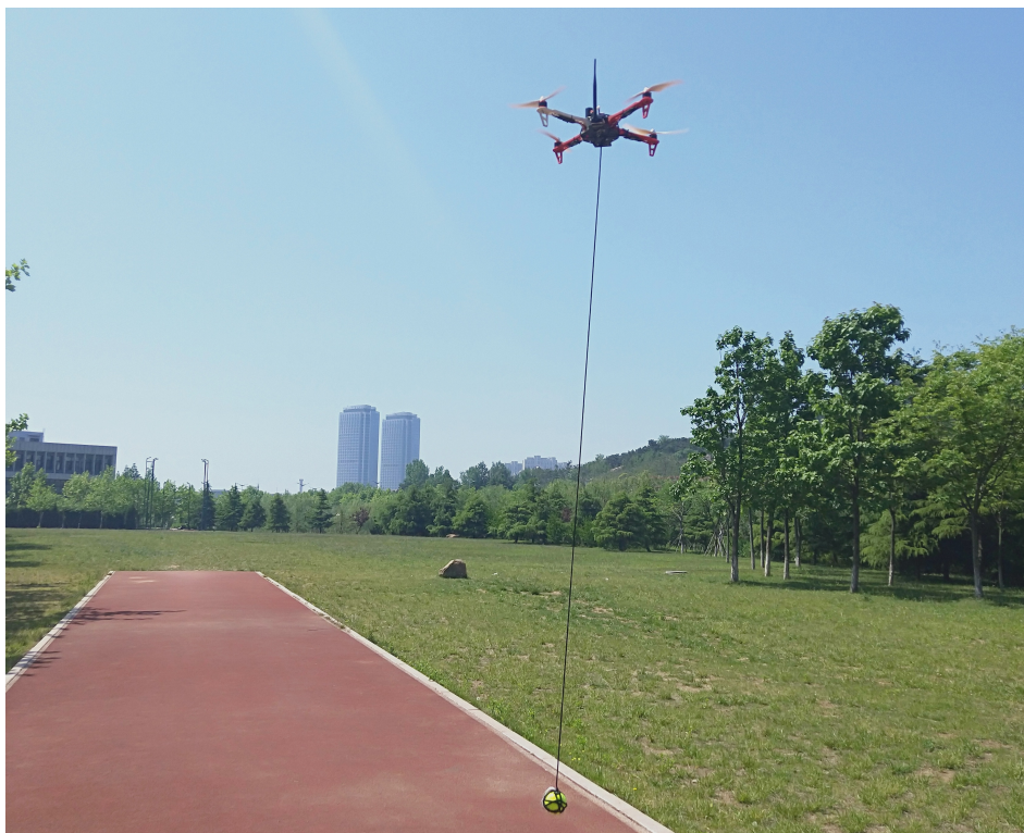
Figure 8. The UAV transportation system following the pre-planned path in the outdoor experiments.
