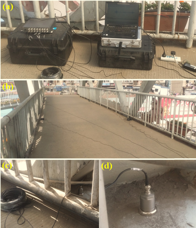
Fig. 6. Experiment configuration: (a) signal conditioning box and laptop implemented with data acquisition software; (b) sensor layout on the bridge deck; (c) sensor connected with shielded cable; (d) sensor fixed close to bottom chord joint through magnetic base.
