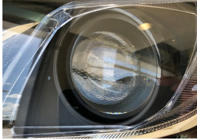
Figure 2. Headlamp lens with tiny texture
