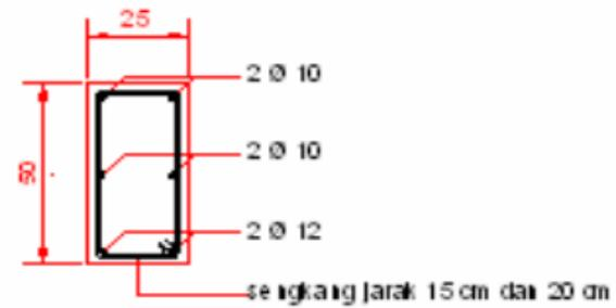
POTONGAN PENULANGAN BALOK A ATAU B
