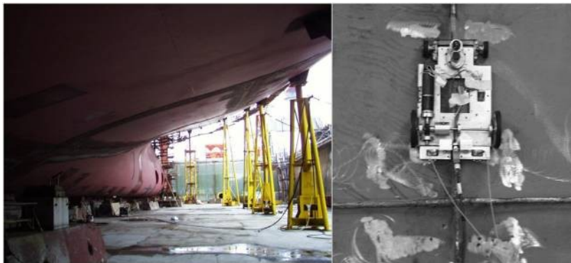
Figure 7. Steep and shallow profiles of stern segment of the hull of a container ship and a magnetic adhesion robot. 6
